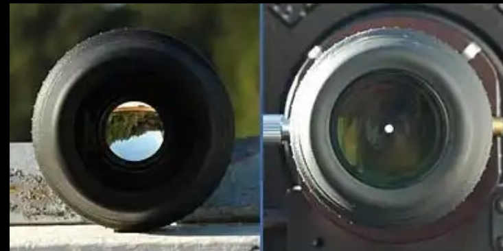
(left) eyepiece exit window; (right) telescope exit pupil
