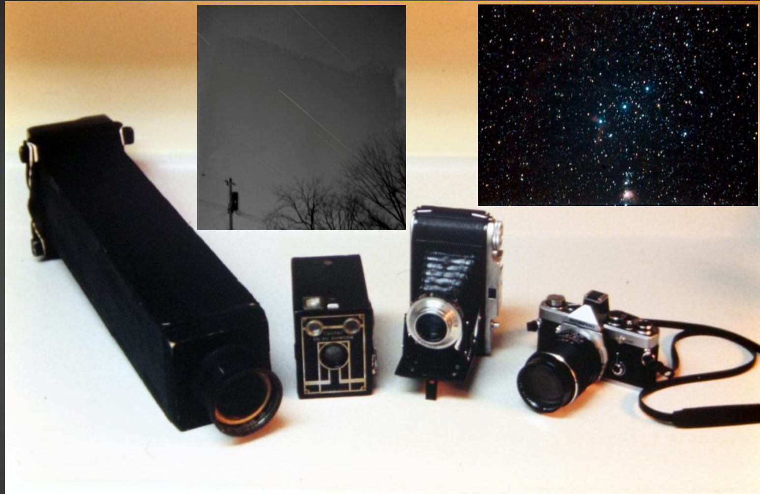
Homebuilt 4x5 Sheet Film Camera 50mm f/11 Refractor Lens (Polaroid Film Back)
